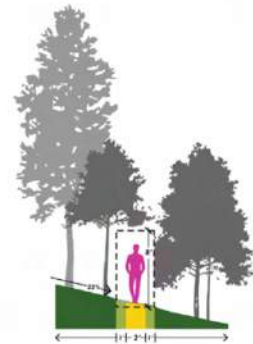
RIDGELINE TRAILS pedestrian only tread width - 2' clearing width - 4' wide 8' high ideal slope - less than 10%
